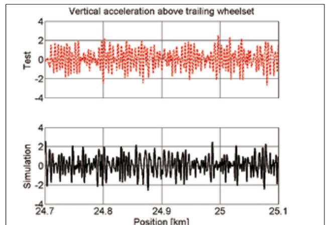
... for two-axle vehicle with link suspension.
