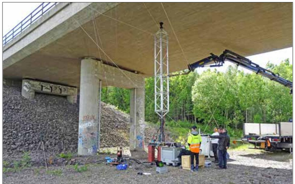
**Pilot testing of a hydraulic bridge exciter developed by KTH.**
