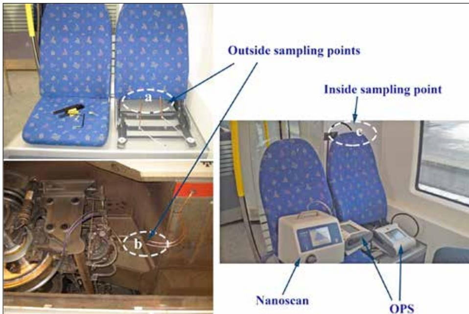
Two sampling points, outside sampling point under the train between two bogies (left a and b), inside sampling point close to passenger's breathing area (right c), attached to particle counters inside the train cabin.
