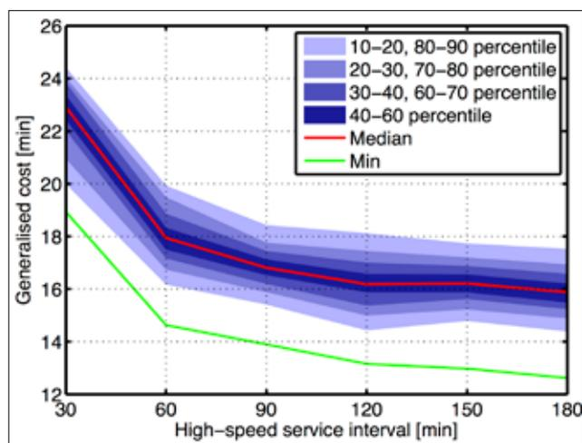
Generalised cost as a function of service interval for the high-speed services on a line with mixed traffic.
