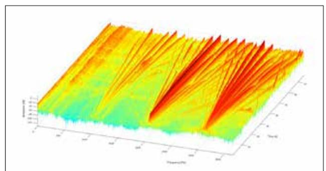
**Noise spectrogram of the tested traction motor during acceleration**
