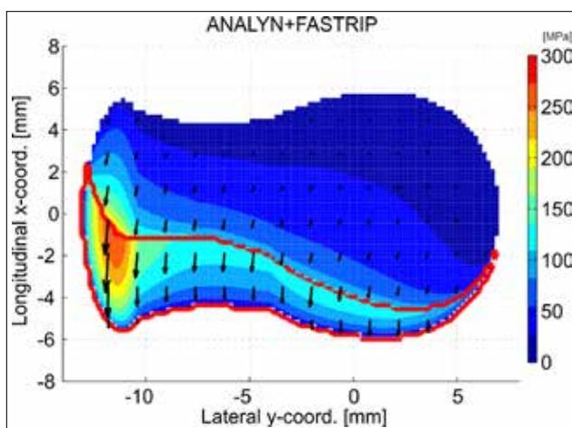
Example of contact patch and tangential stress distribution (magnitude, direction). The red line encircles the slip part of the patch.
