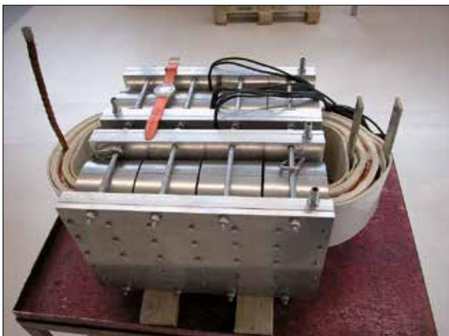
Prototype of medium frequency transformer for 200 kVA, 4 kHz.
