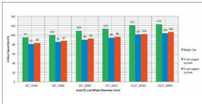
Comparison of critical speeds for different vehicle configurations.
