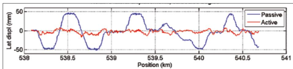
**Relative lateral displacement between carbody and bogie with and without active lateral suspension.**
