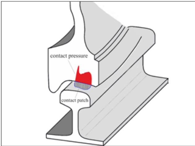
**Example of half contact patch (grey) and pressure distribution across the patch at longitudinal mid-position (red).**
