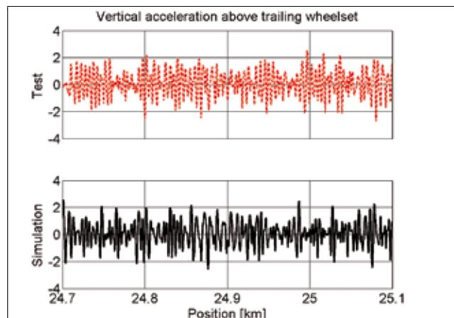
... for two-axle vehicle with link suspension.
