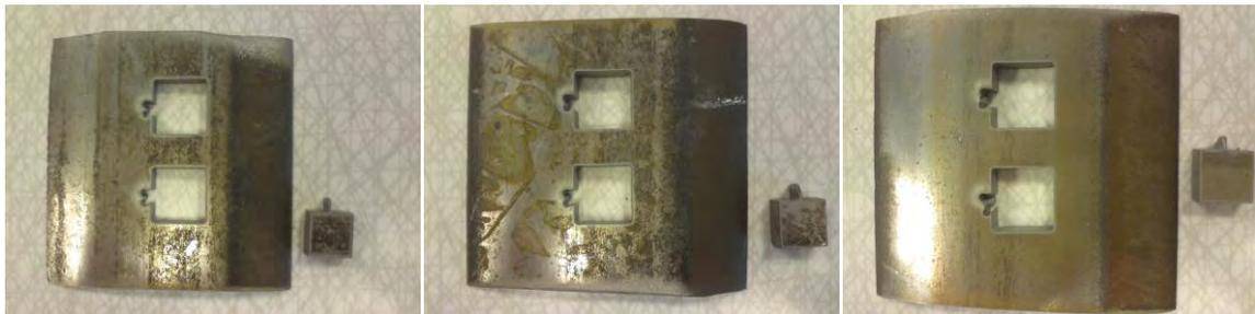
**Fig. 2.** Rail section samples, showing: left, blackish layer; middle, leaf residue layer; right, uncontaminated surface.
