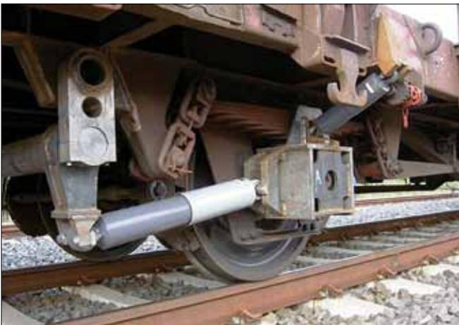
**A two-axle wagon with different damper arrangements was successfully tested at speeds up to 176 km/h.**
